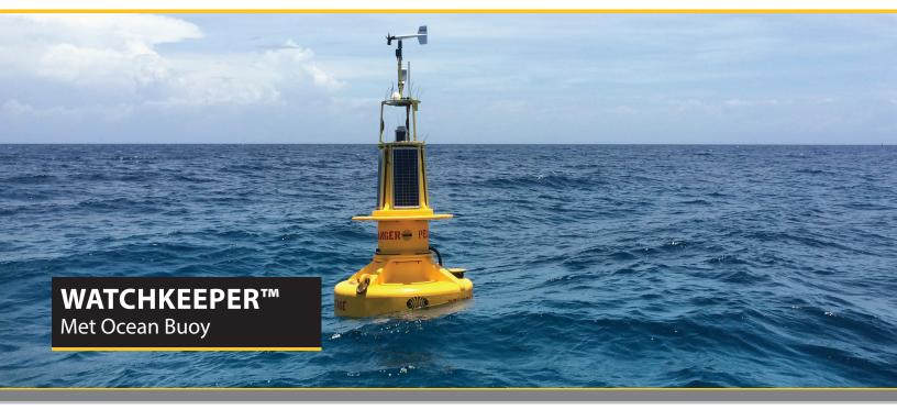
The WatchKeeper<sup>™</sup> Met Ocean Buoy is a versatile data collection buoy for large lakes, rivers, harbours, and coastal water deployments.
